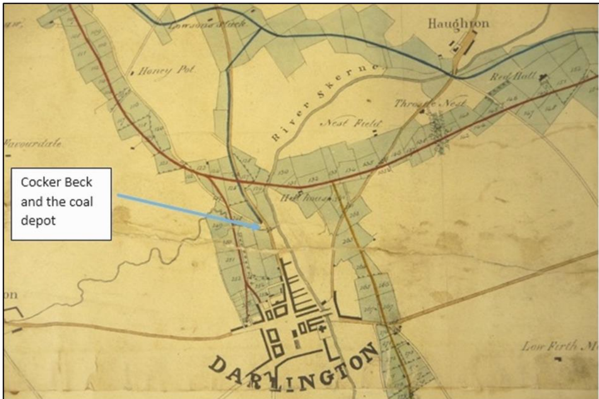
Figure 6. The proposed branch line from the main line into Darlington as set out by Stephenson in 1823 (shown as a red line) and Overton in 1821 (shown as a dark blue line). Unusually, the branch line in the end followed Overton's route, which terminated at Cocker Beck, not Stephenson's route which extended into the old town.
