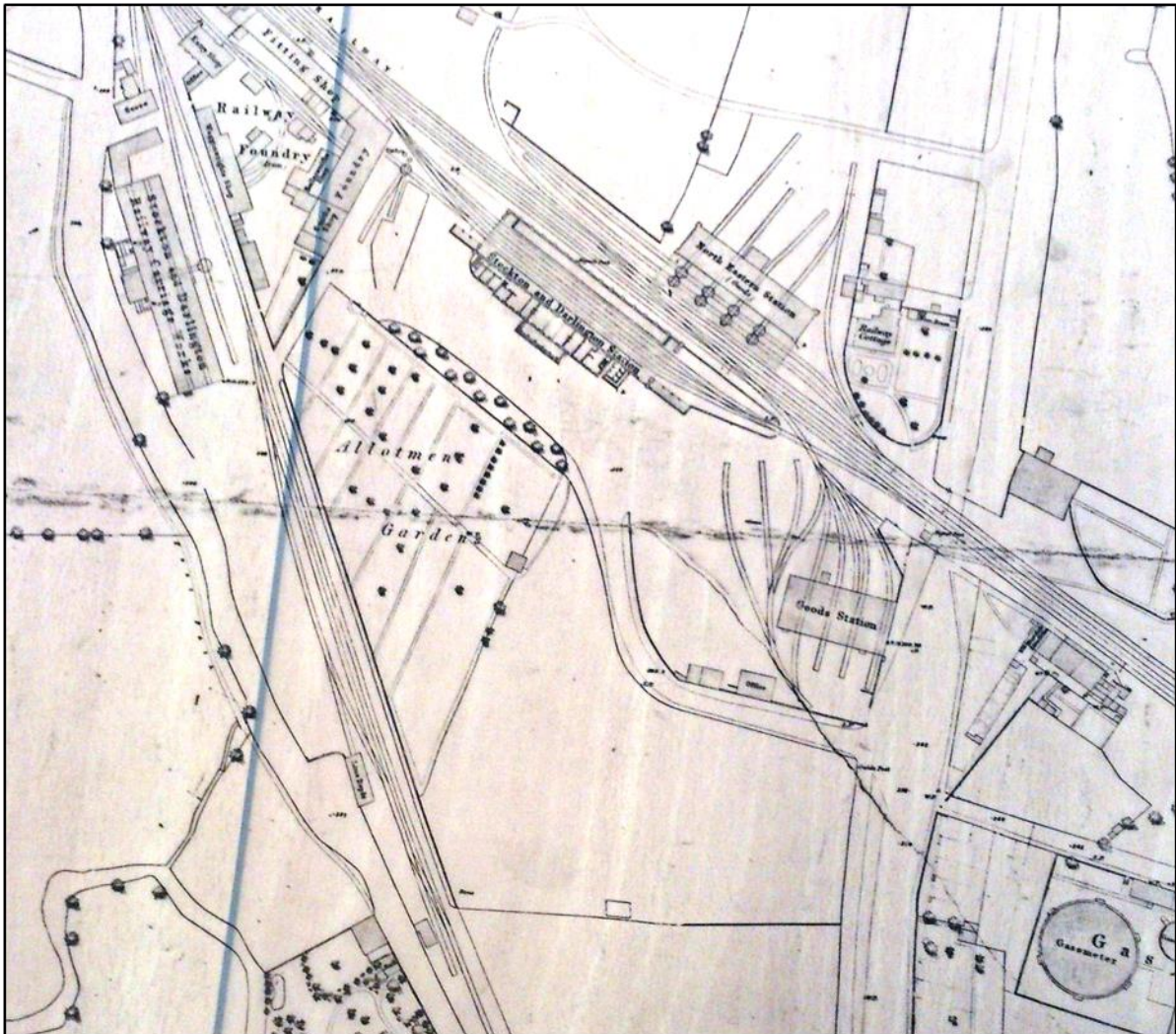
Figure 5. The S&DR North Road station shown on the 25" to 1 mile 1 st ed OS map of 1856 (surveyed 1855) on the south side of the tracks. Kitching's Railway Foundry is located to the west, and the S&DR Goods Station and Offices on McNay Street are also shown. The S&DR Carriage works can be seen with a turntable to the front and sidings that go on the lime depot. The original (and first) purpose built station can be seen on the east side of North Road but is not annotated, presumably because it was now used as cottages for railway staff and their families.
