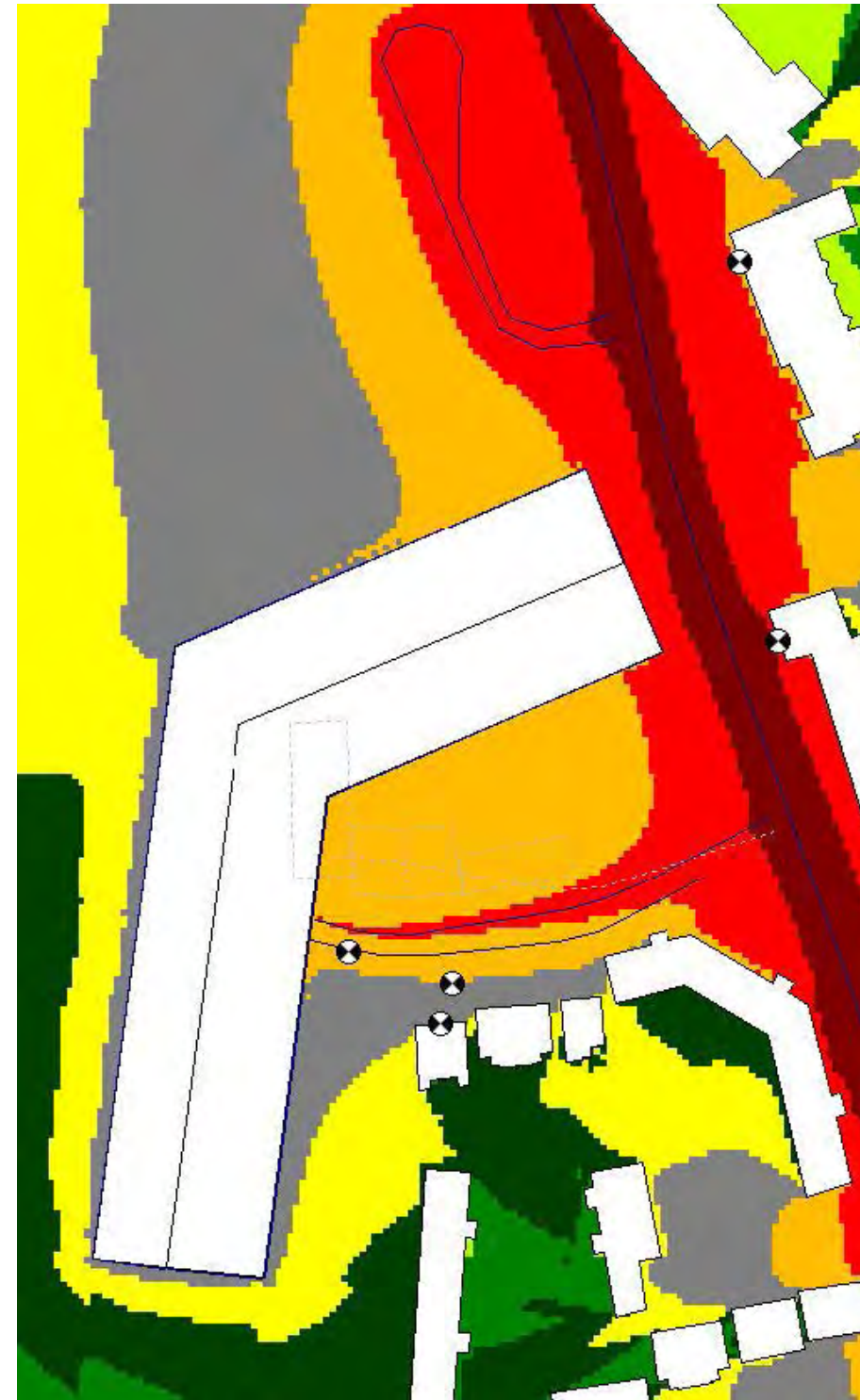
Scenario 1, noise contours at 4m showing the AM ambient noise level Diagram taken from Stroma Planning Acoustic Assessment
