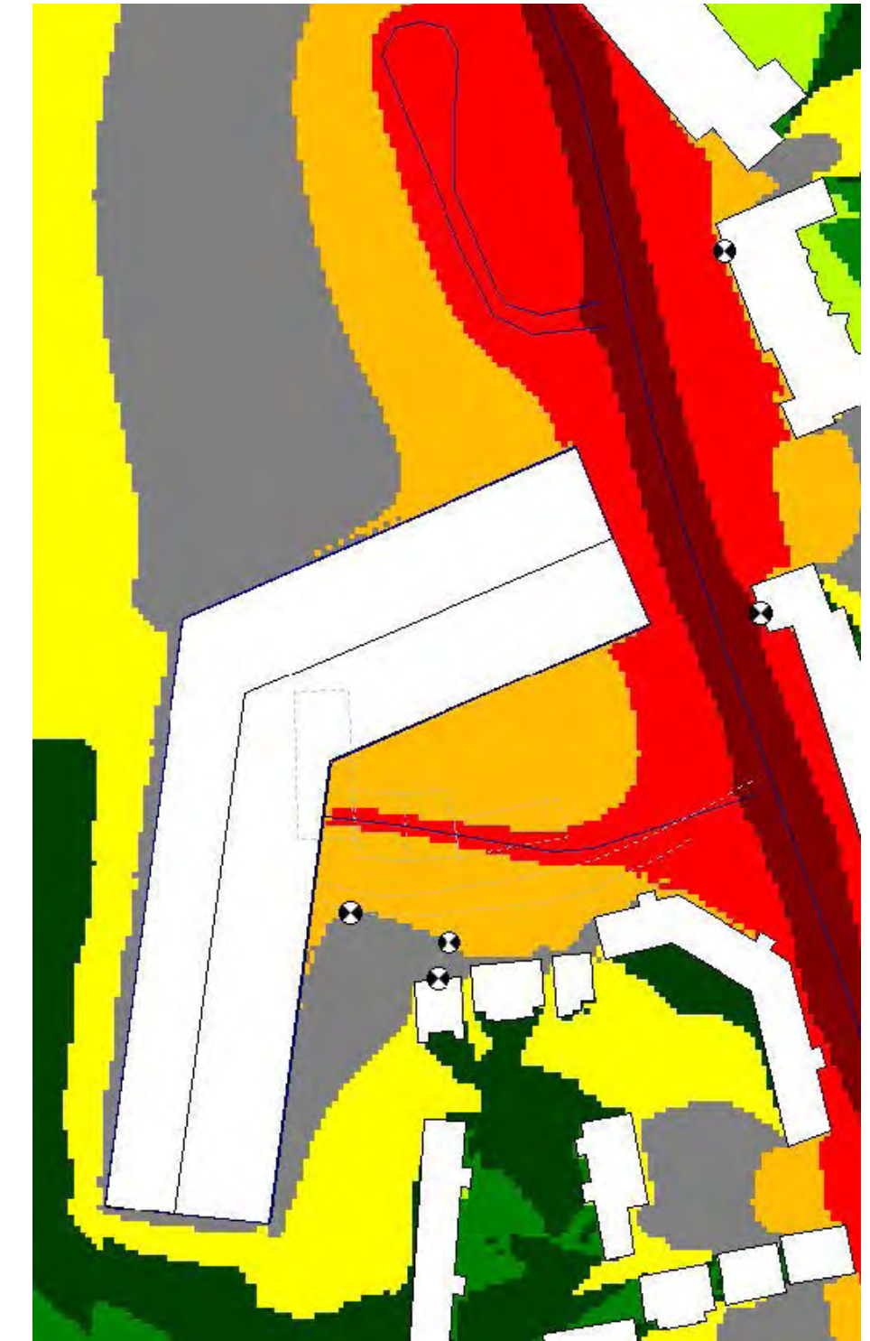
Scenario 2, noise contours at 4m showing the AM ambient noise level Diagram taken from Stroma Planning Acoustic Assessment
