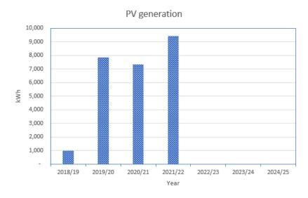
In 2021/22, 9,440 kWh of electricity was generated by our solar panels. The increase is, in part, due to the additional capacity that has been added to the Town Hall roof. Generation can never be guaranteed as it is so weather dependent.
